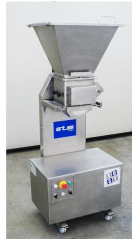
The granulating machine (GTS) has been designed for granulate solid food products continuously. The product is introduced into the hopper and then carried to special rotary blades, that process the product in granules. The granulating machine has a loading platform, where you can place the baskets for collection; alternatively, the handles are suitable for the anchoring of bags.
